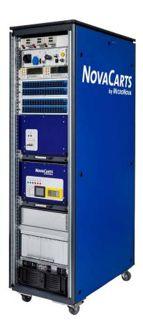
**3** NovaCarts HiL System for the testing of battery management Systems
