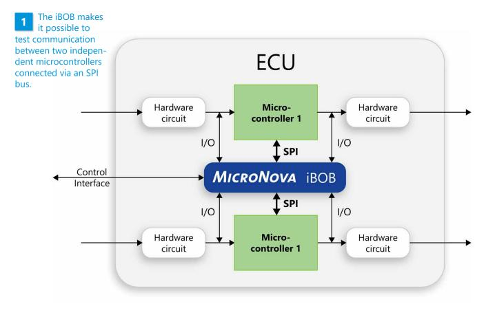
As well as recording data, the iBOB also enables the manipulation of signals to test the error behavior of masters and slaves or the error algorithms, for example. Messages can be varied in nine different selectable ways. The data can also be manipulated,
