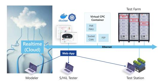
The basic principle of NovaCarts Virtual is a networked real-time cloud.
