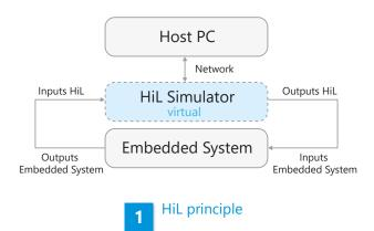
In addition, NovaCarts Virtual as a virtual real-time computer can also be used to carry out a lot of preparatory work for the real HiL test. Optimized preparation helps to use the limited resources on the HiL simulators as efficiently as possible.
